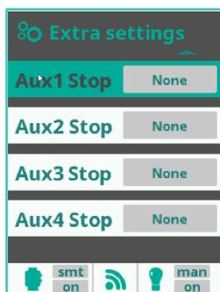
Here it can be defined for the relays Aux1 to Aux4 whether the switching on of the respective relay is interrupted by the occurrence of the alarms FL1 and/or FL2.
