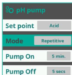
Setting "Mode": **Repetitive** => Adjustment option of the pump operation time:
